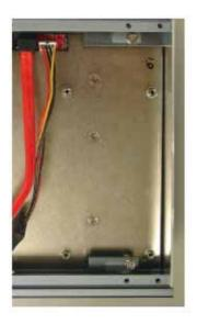
4. Put the HDD into the HDD Holder Bracket and screw it on.
